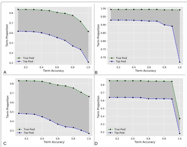
**Fig. 7** Labor automation analysis. **A** Fraction of labels identified by the metadata extraction system across all metadata categories as a function of identification accuracy. The green curves represent all suggested terms regardless of rank (True Pool), while the blue curves represented the recommended terms only if they appear at the highest rank (Top Pool). Same analysis broken down by species (**B**), brain region (**C**), and experimental condition (**D**)
