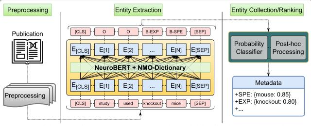
**Fig. 3** Overview of the architecture of the metadata extraction system used in this study. The full text of the publication is preprocessed, marked with sentence boundaries (CLS and SEP), and converted into sequences of words. Each sequence is then passed through the entity extraction algorithm to identify occurrences of metadata entities. The candidate terms are then post-processed and ranked based on relevance score
