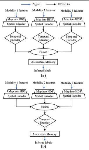
**Fig. 3** HDC **a** late fusion and **b** early fusion architectures for a three-modality emotion recognition system. The late fusion architecture fuses after the temporal encoder, resulting in 3 parallel temporal encoders—one per modality. In comparison, the early fusion architecture fuses before the temporal encoder, resulting in only 1 temporal encoder
