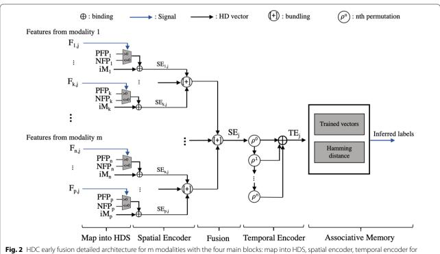
Fig. 2 HDC early fusion detailed architecture for m modalities with the four main blocks: map into HDS, spatial encoder, temporal encoder for n-gram of size n+1, and associative memory. Sensor fusion occurs early in the datapath, directly after the spatial encoder
