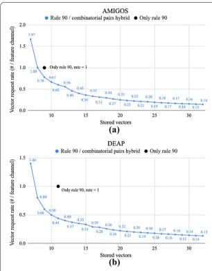
**Fig. 8** Vector request rate (number of vectors requested per input channel) as the number of vectors stored increases while using rule 90 on a small set of continuously re-populating vectors as compared to only rule 90 for **a** AMIGOS and **b** DEAP
