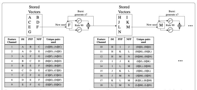
**Fig. 5** 'Combinatorial pairs' feature channel vector set generation demonstrated for 7 stored vectors. iM loops through vector bank after exhausting available sequential pairs for FP. Hybrid method follows by burst re-generating the vector bank with rule 90 so that new combinatorial pairs can be formed for more feature channels. Generation of 18 feature channel vector sets using a bank of only 7 vectors is shown
