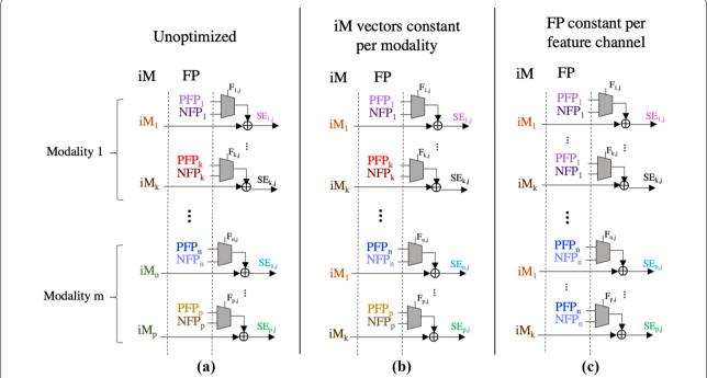
**Fig. 4** iM and FP vectors used to map into HDS to generate unique SE vectors per channel for **a** 'unoptimized' with distinct iM and FP vectors for all channels, **b** 'iM vectors constant per modality' with the same iM vectors between different modalities, and **c** 'FP constant per feature channel' with the same FP vectors between channels of the same modality
