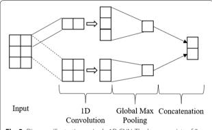
**Fig. 3** Diagram illustrating a single 1D CNN. The layer consists of 2 filters of size 1 and 2, respectively
