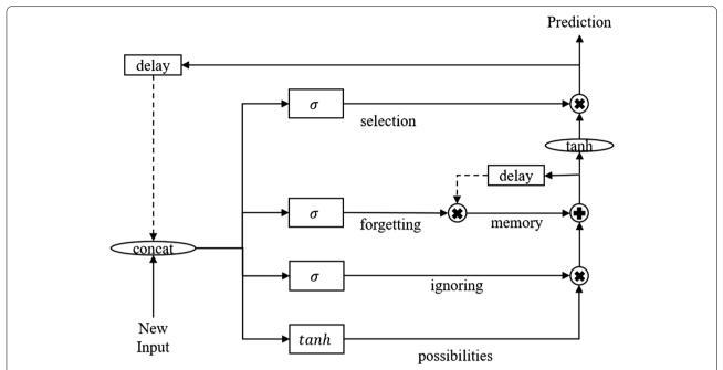
**Fig. 5** Diagram illustrating the LSTM architecture. The tanh and  $\sigma$  gates are hidden layers with sigmoid activation function, + and x connections are pair-wise addition and multiplication operators, respectively. At the same time, the || connections are vector concatenation operators
