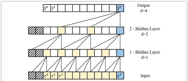
**Fig. 8** Diagram rendered from [58] illustrating dilated casual convolution layers from of filter size 3 and increase dilation of (1, 2, 4). At the second hidden layer, a neurons field of view is 6 (i.e., its scope allows it two see up to 6 input sequence within the past)
