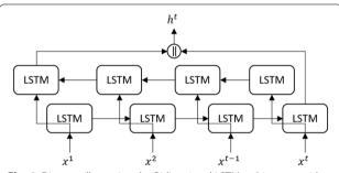
**Fig. 6** Diagram illustrating the Bidirectional LSTM architecture with the standard LSTM cell, as illustrated in Fig. 4
