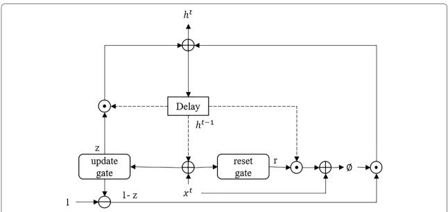
**Fig. 7** Diagram illustrating the GRU architecture. The reset and update gate are hidden layers with sigmoid activation function, + and x connections are pair-wise addition and multiplication operators, respectively. At the same time, the || connections are vector concatenation operators
