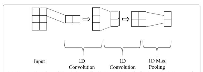
**Fig. 4** Diagram illustrating a 2-layer stack 1D convolution network. The first 1D convolution has 1 filter of size 1, generating a 3 - 1 feature map. A second convolution takes the 3 - 1 feature map and applies a 1D convolution with 2 filters of size 2, generating a 2 - 2 feature map. 1D max Pooling is then applied after the second convolution producing a vector
